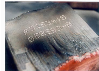
INFODENT® permanent mechanical marking
