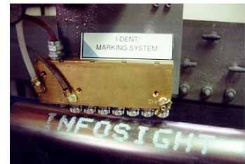
I-DENT® Automatic ink spray marking
