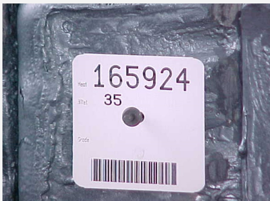
InfoTag® nailed to cast steel.
