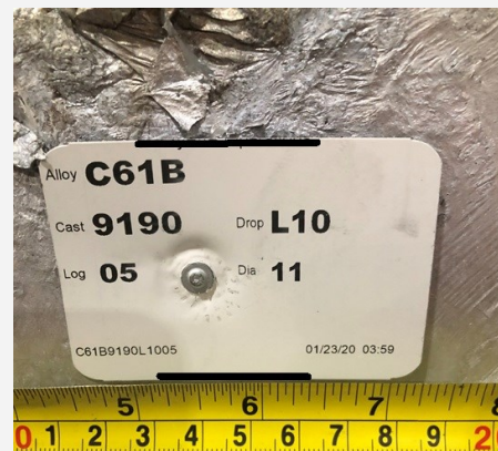
AlumaTag™ nailed to cast aluminum.
