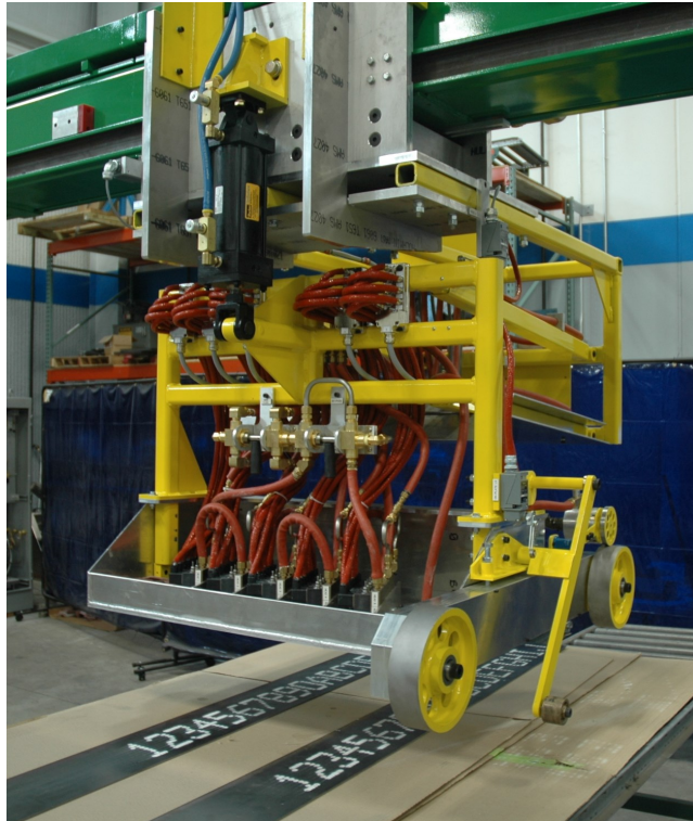
Typical 5-head marking carriage
