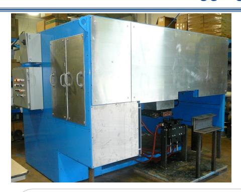
The InfoSight Model 2900 automatic single station slab tagging for stationary system slabs is the ideal bar code tag solution when it comes to MIG-welded tag identification of carbon steel slabs with high contrast marking.
