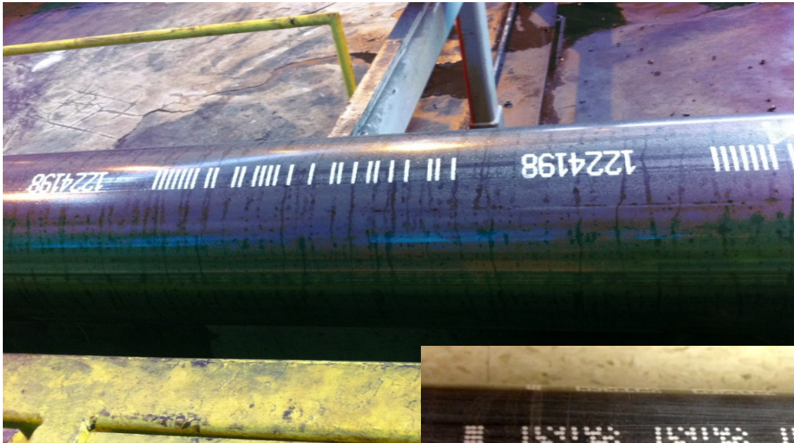
Typical 27 bar OC™ bar code on pipe OD— approx. 18"W x 1.25"H (457mmW x 32mmH)
