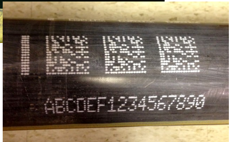
Typical redundant 2D bar codes on pipe OD—each approx. 1.25" square (32mm square)
