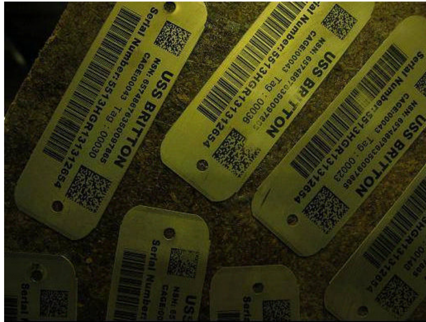
Figure 9. View of LabelLase® Damage after an Abrasion Run
