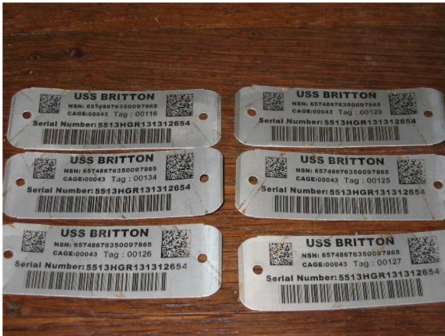
Figure 13. Impact damage to tags after impact from three weights
