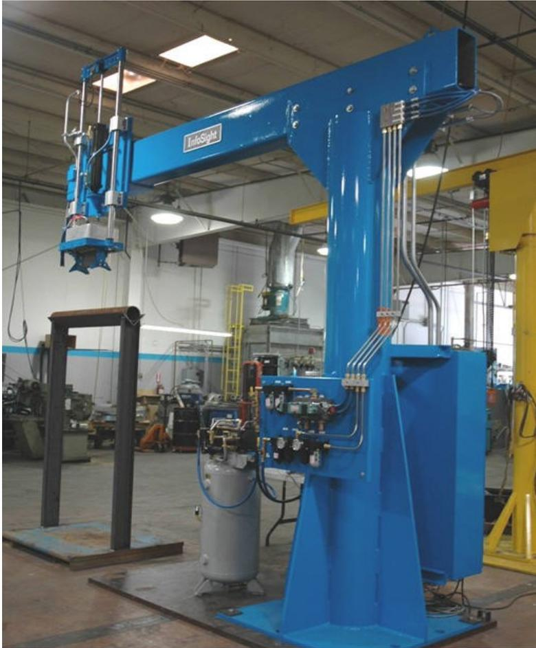
**Typical Jib Stamping System for pipe**
